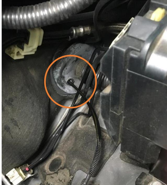
6. Once the water sensor harness is inside the vehicle, neatly route the cable under the dash to driver's side of the vehicle. Ideally located near the fuse panel.
