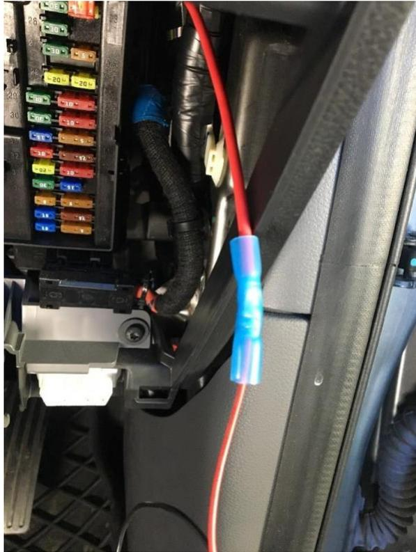
9. Identify a fuse in the factory fuse panel that can be used to install the add-a-circuit. It is recommended to use a fuse/circuit that is switched with either the accessories or ignition e.g., Cigarette fuse.
