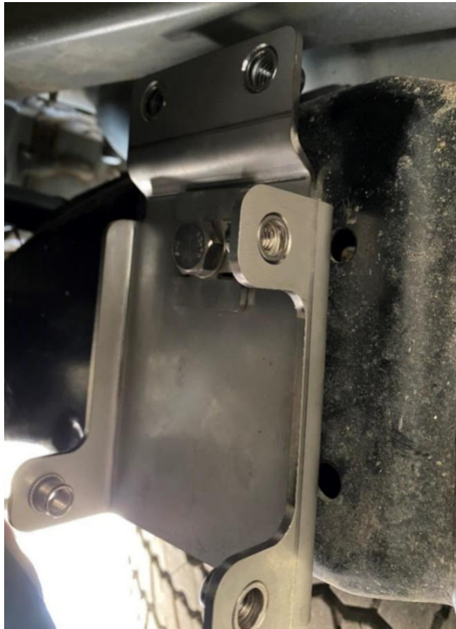
DP Ryco bracket secured in place, note how smaller bracket lock in to prevent movement from the main bracket
