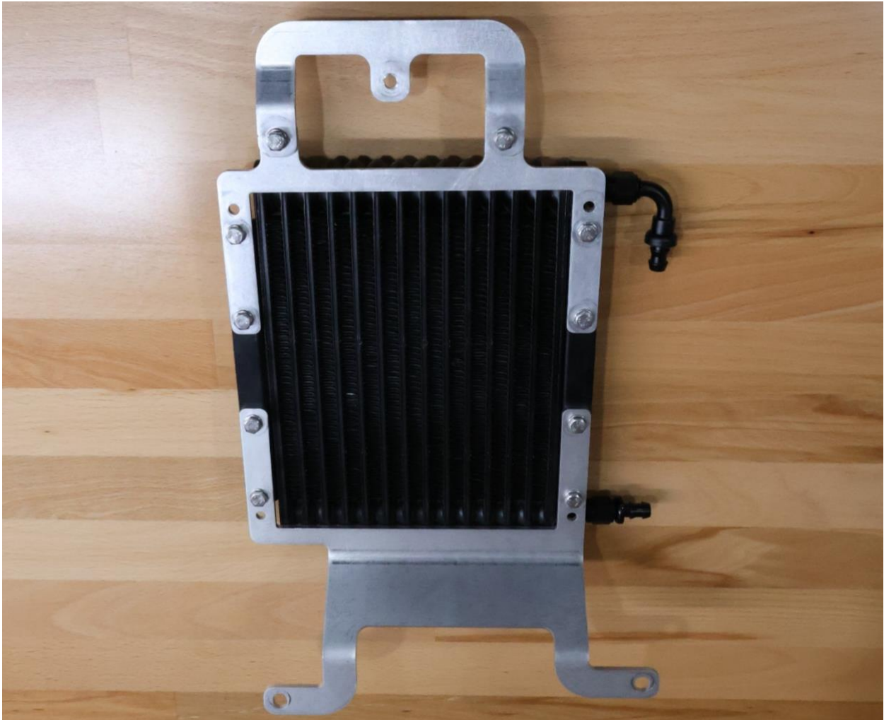
Cooler assembly with fittings in place at correct orientation
